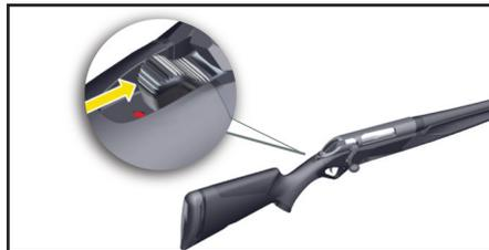
2. Make sure that the **rifle** is cocked: the red dot on the cocking piece at the end of the upper receiver is visible.
