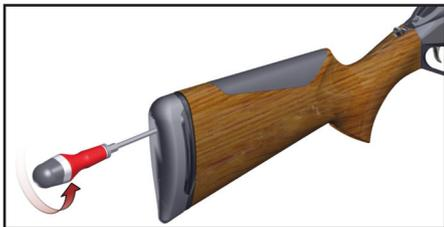
**Caution:** In order not to damage the recoil pad, **spread** the tip of the screwdriver with Vaseline or other grease.
