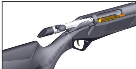
3. Return the **bolt to the closed position (a-b)**. Verify empty chamber and close bolt.
