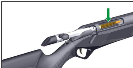
Closing the bolt manually will chamber the first cartridge from the magazine, leaving the rifle ready to shoot.
