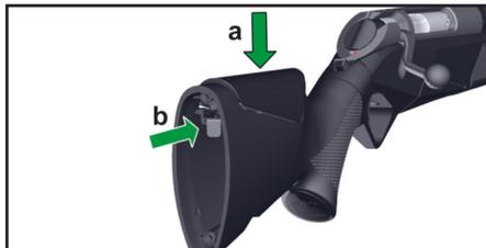
**Caution:** the comb, when correctly fitted, is aligned seamlessly with the outer edge of the stock.
