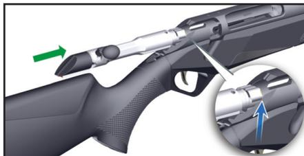
3. Slide the **bolt** forwards and turn it with the **lever** until the bolt is closed.
