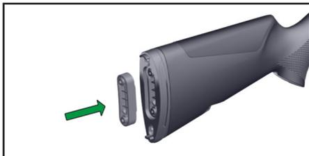
6. Refit the **recoil pad "1"** and fasten it with the two screws in the KIT, taking care to use the **medium-length** screws for one pair of shims, or the **longest screws** for two pairs (Phillips screwdriver, recommended tightening torque **2 Nm**).
