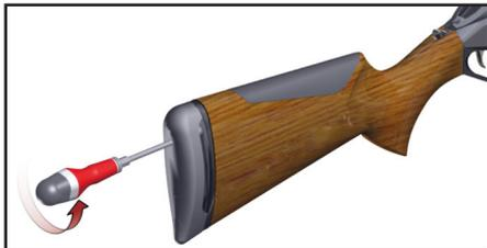
**Caution:** In order not to damage the recoil pad, **spread** the tip of the screwdriver with Vaseline or other grease.
