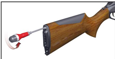
3. Using an Allen key, work from inside the stock to remove the **rubber cap** from the hole for the sling swivel.
