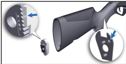
**Caution:** in case of RH/LH stock deflection, the **locking plate** to be used must be positioned with the chosen stamped side facing the butt plate.
